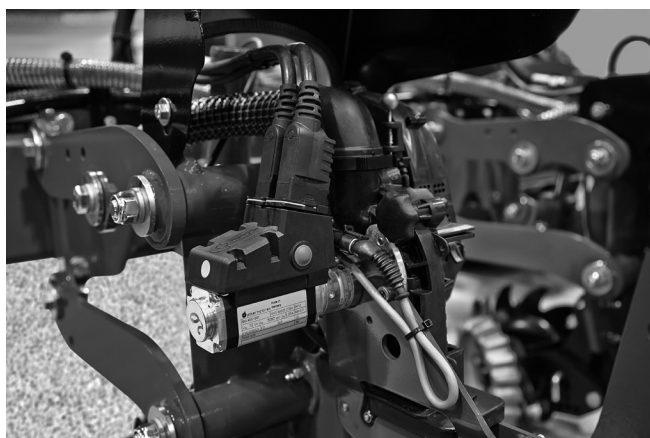
Figure 4. Planter row unit with electric seed meter.
